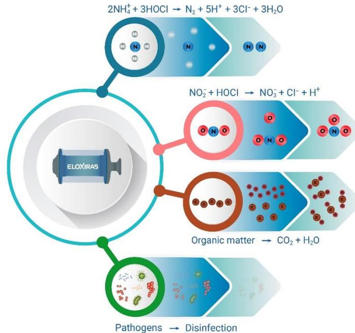
Figure 2. Main electrochemical reactions produced in ELOXIRAS®.
