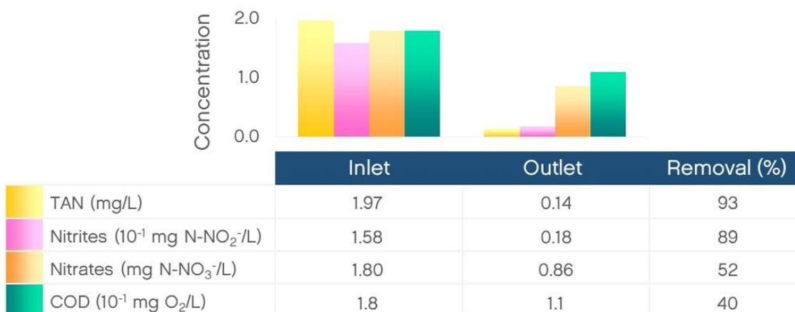
Figure 4. Experimental values of key pollutants at the inlet/outlet of the ELOXIRAS® system.
